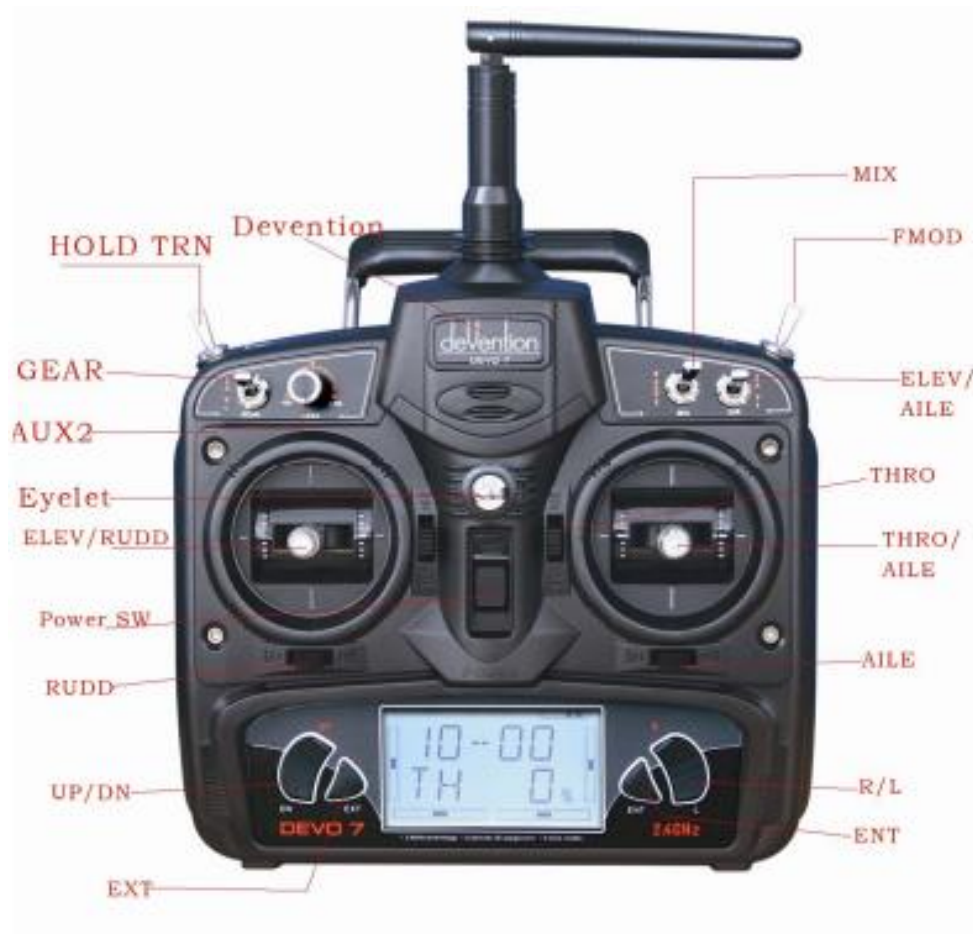
Figure 1: The DEVO 7 transmitter with buttons labeled.
