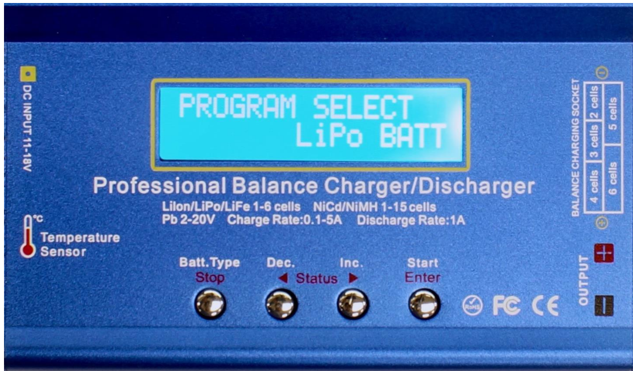
Figure 3: Set program select to LiPo Battery.
