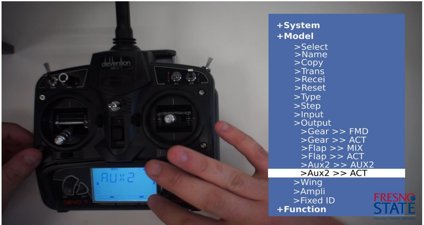
Figure 4: Transmitter settings for the output menu.
