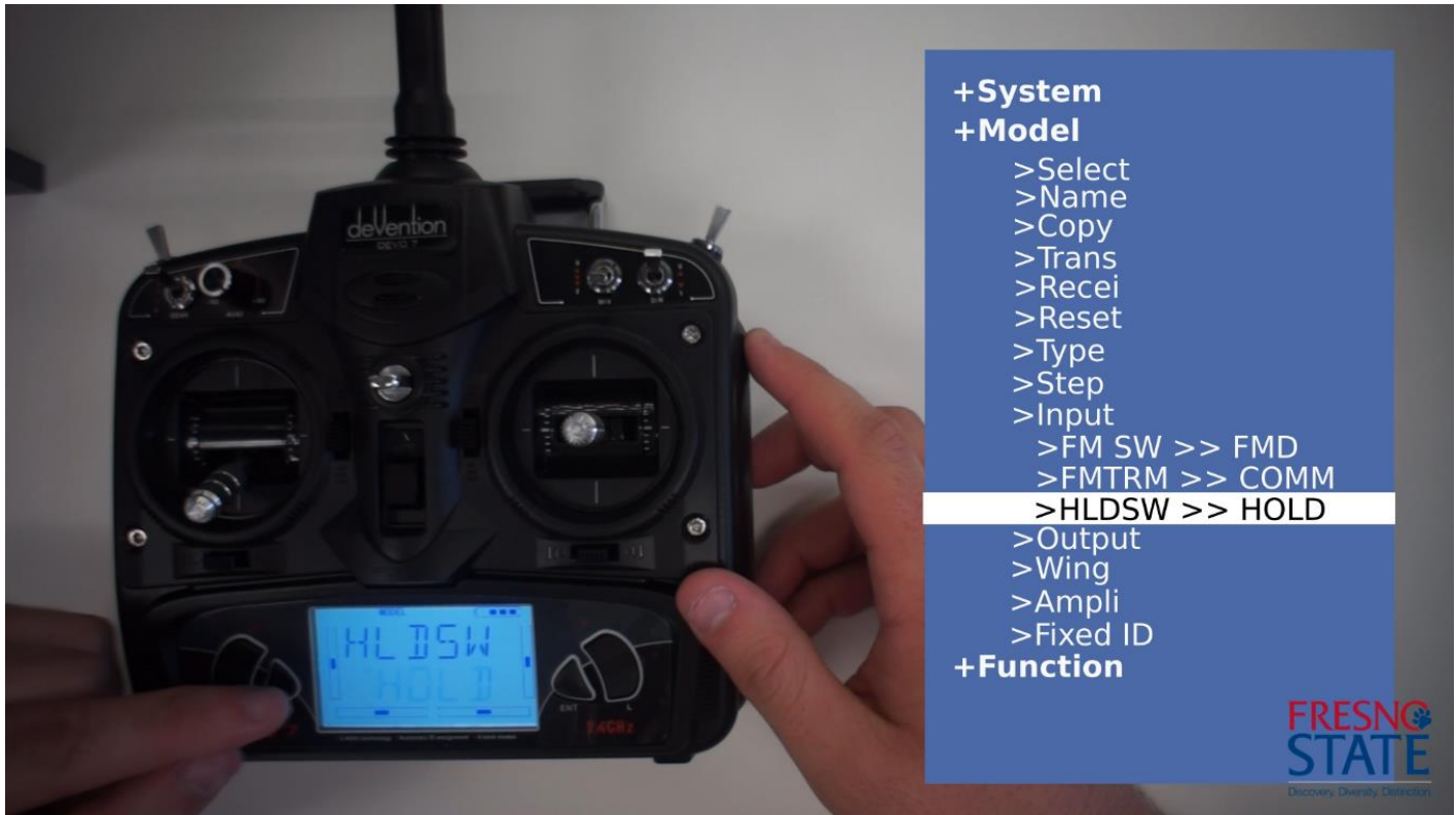
Figure 3: Transmitter settings for “ FM SW ”, “ FMTRM ”, and “ HLDSW ”.
