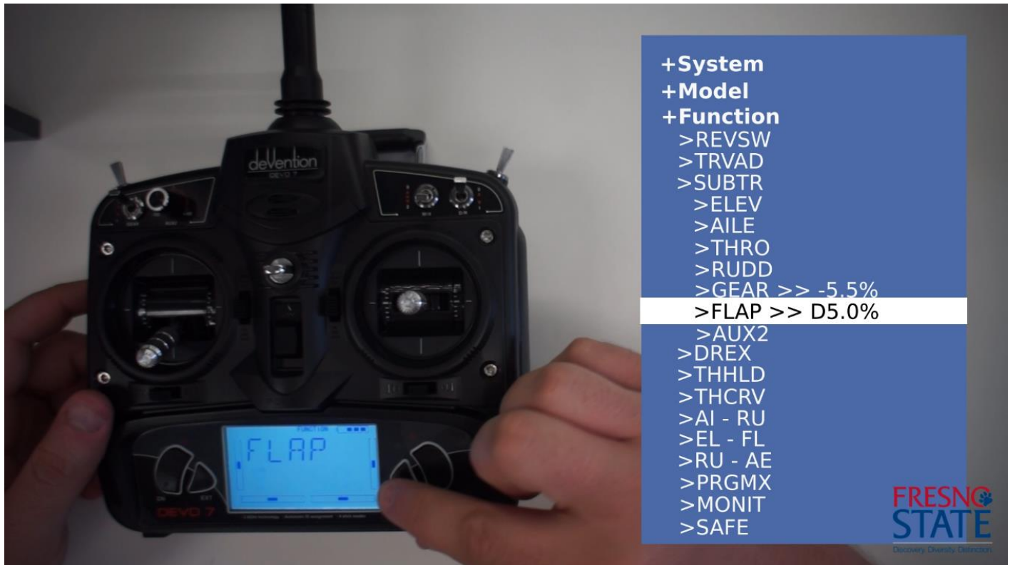
Figure 8: Transmitter settings for “ SUBTR ”.
