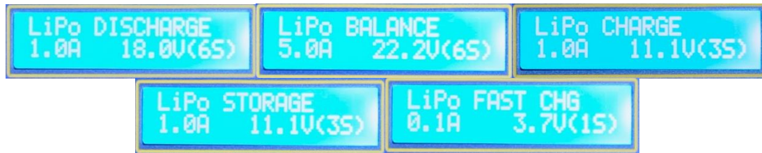
Figure 4: Charging and discharging options.
