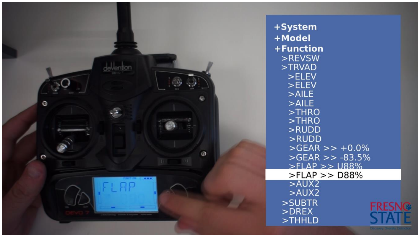
Figure 7: Transmitter settings for “ TRVAD ”.
