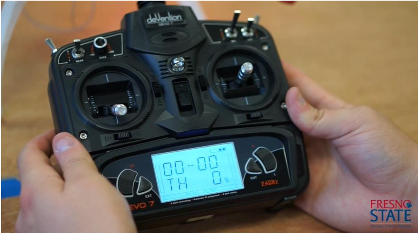
Figure 13: The transmitter is ready to set a fixed ID for the receiver.
